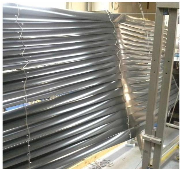
According to EN1932:2013 methodology the blind is covered with plastic film, put in frame and exposed to air blow strain. The plastic film prevents from air pressure decrease caused by air flowing around and between slats. The new method is closer to real conditions to which the blinds are exposed.
